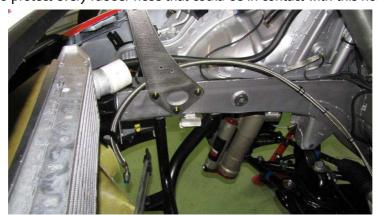
Protect as much as possible the wiring looms and other hoses (Lambda sensor, fuel hose, water hose...) that can be close to the exhaust line using the appropriate thermal protection.
